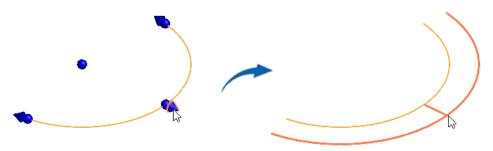
You can lengthen or shrink the arc using the conical handles on the end points. The diameter remains intact.
