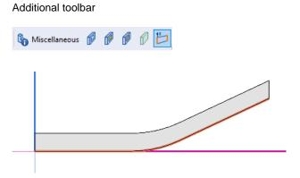
When the function is turned off, the blend is created with its end faces orthogonal to the path.
