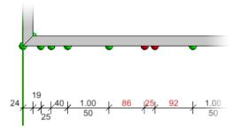
A notice will appear in the status bar showing the quantity of the defective dimension chains and the dimension points that are no longer connected.
