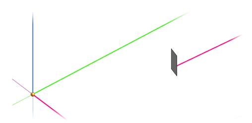
When off, the function is inserted orthogonally to the path.
