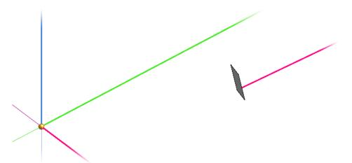
The **Blend** function has also been expanded by a function. By turning on the new icon **End faces parallel to the global z-axis**, the blend is generated with its end faces parallel to the z-axis.
