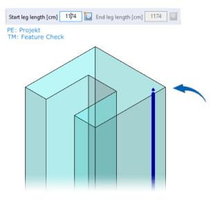
When you click in the end portion length edit box, the selection moves to the other side of the bending shape. When the hook is input, this visual indication is also automatically displayed at the end of the bending shape to which the active input in the additional toolbar relates.
